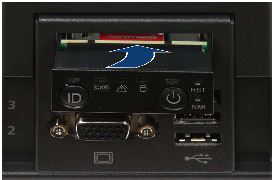
Figure 196: Installing the control panel
